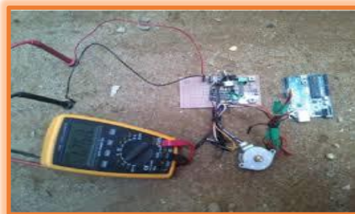
Figure 82 Automatic valve regulation circuit.
